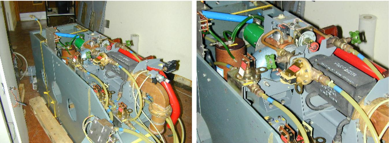
Even though the interconnections between the basic components in the linac's radiofrequency system are straightforward, we all know that it is easier to take apart than to put together again. Reverse-engineering a complex bit of kit can be full of unexpected surprises. So detailed, very detailed and very, very detailed pictures are always a good idea. Here is a selection showing the magnetron, the isolator and the output waveguide.
