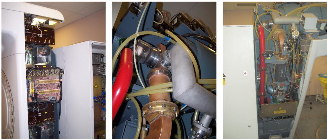
Details of the accelerator: The focus supplies on the left, the gun, mode transformer and vacuum pump in the middle and the radiofrequency generator on the right.
