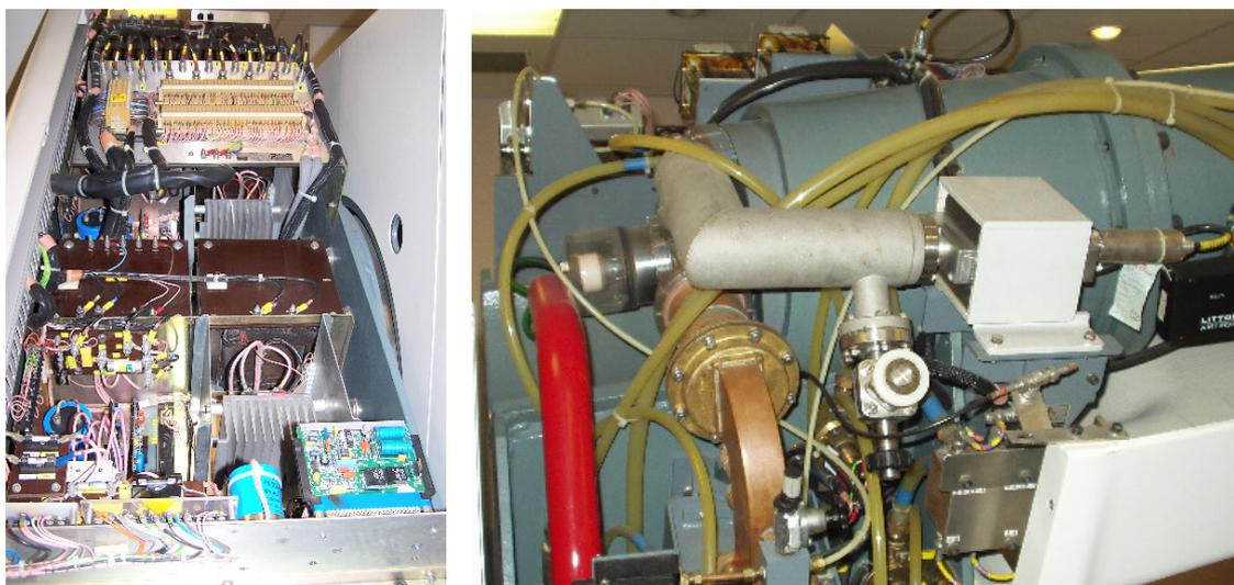
Details of the accelerator: The gun and magnetron drive circuits on the left and details of the gun assembly on the right.
