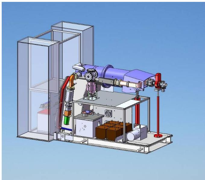
SolidWorks designs: the elevation and isometric views of the machine. At this stage ‘bits’ can be readily re-positioned, and it is easy to forget that we are dealing with structures weighing several tons in total.
