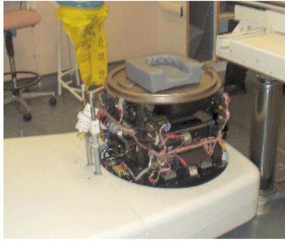
The head assembly, inside which is the x-ray target. This, at least, is one complex item which we will not need.
